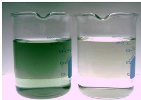
After electrocoagulation the water is treated by a filtration step removing the suspended solids. The filtered water can be reused. When required, the dissolved solids are removed in a succeeding reversal osmosis step to produce water with a high quality.
